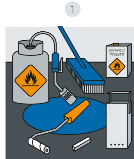
Equipment: Torch, broom, piece of chalk and drop-on material. Use a primer if necessary.
