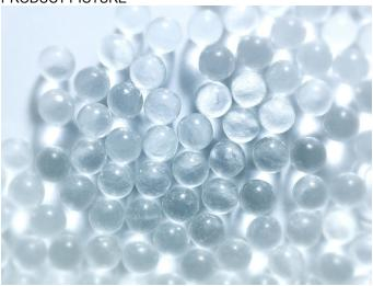
The retroreflective glass beads are engineered to provide high retroreflection. They can be optionally coated with organosilanes to improve bonding with the marking material and thus increasing the durability of road markings. Furthermore, SWARCOFLEX beads can be intermixed with anti-skid particles upon customer request to enhance road safety by improving skid resistance.
