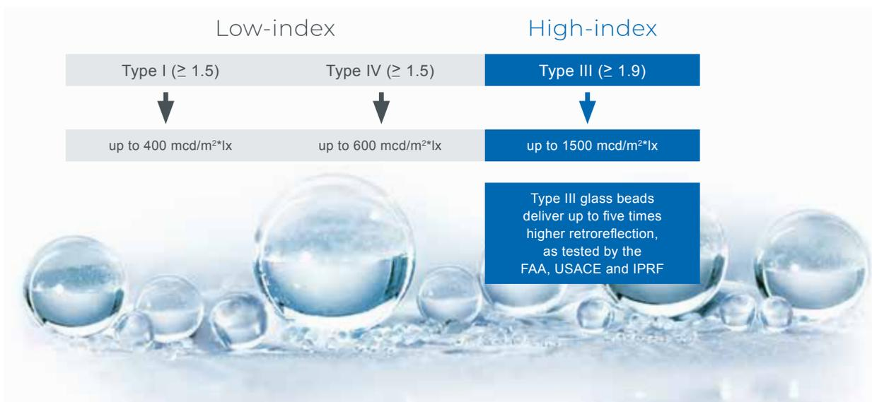
The only difference between type I and IV beads is their size, which also influences their retroreflective values. Type I beads reach up to 400 mcd/m<sup>2</sup>·lx. Type IV glass beads are larger than type I beads, with retroreflective values reaching up to 600 mcd/m<sup>2</sup>·lx. Type III glass beads are high-index beads. These have better optical properties and significantly higher retroreflective values of up to 1500 mcd/m<sup>2</sup>·lx because they are made from special high-grade glass.
